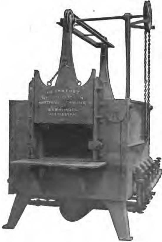
Fig. 194. Large Size Furnace for Heating, Annealing, and Carbonizing Courtesy of Strong, Carlisle and Hammond Company, Cleveland, Ohio
